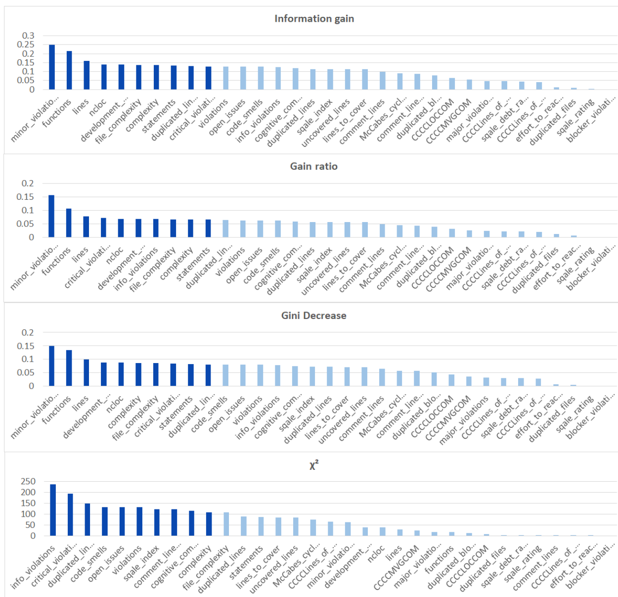
Figure 5. Feature ranks obtained using different types of metrics for the CWE-399 subset of the dataset.
